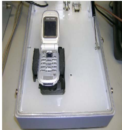
Fig.2 Position of the phone in to the Rohde&Schwarz holder.
